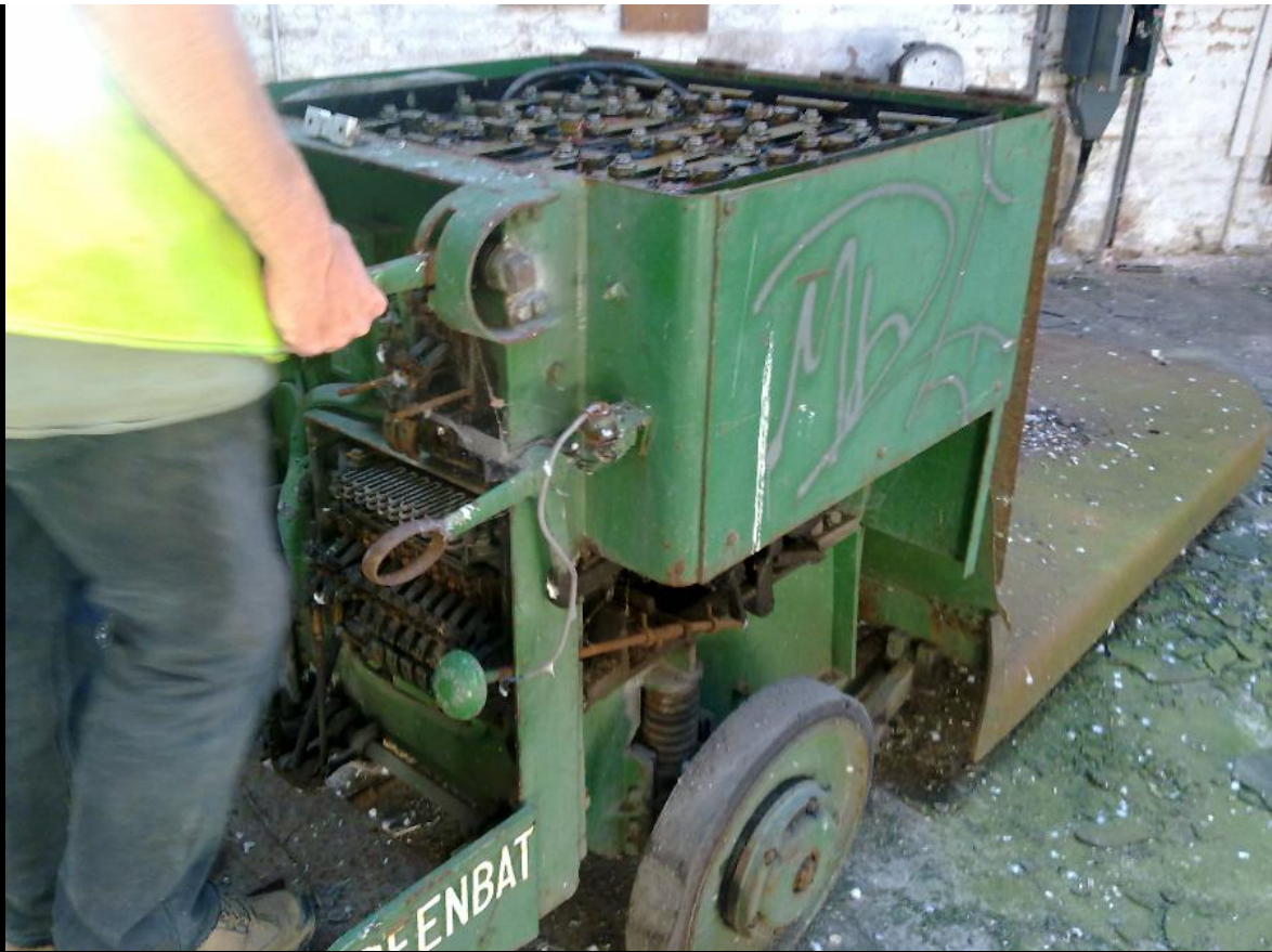
ABOVE & BELOW: The huge amount of batteries needed to power the thing, also Agent Skyframe demonstrating the control gear. This funny little machine had its own handbrake (in hand), direction lever below and emergency stop button (the domed push button at the bottom of the three). It also had working headlights and a horn or claxon. Note the massive row of contactors .
